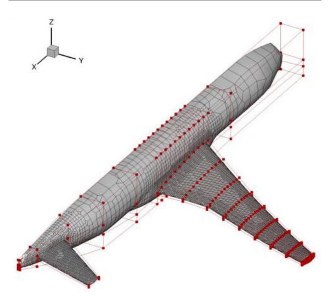
We use the OpenFOAM's built-in mesh tool snappyHexMesh to generate the unstructured hexa mesh. We use ICEM to generate the body-fitted FFD points. We define two more global design variables: twist and tailTwist:
