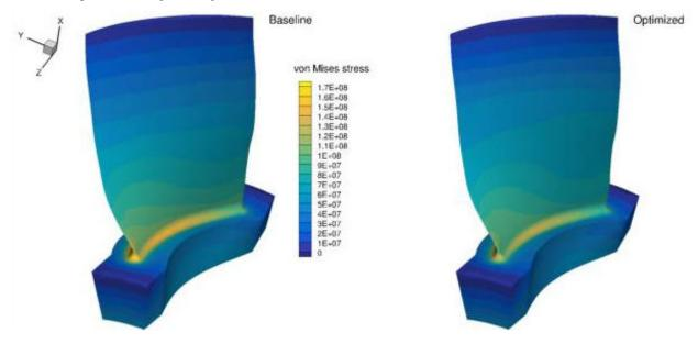
We use solidDisplacementDAFoam. The mesh and FFD setup are same as *Axial compressor rotor*. The rotor runs at 1860 rad/s.
