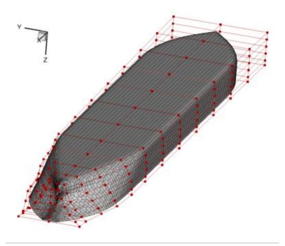
The runScript.py is written for multi objectives configurations where we can combine drag and wake distortion. In this case, the weight for wake distortion is set to be 0. We need to use more refined mesh to obtain an accurate wake distortion value. We also have a curvature constraint for this case.
